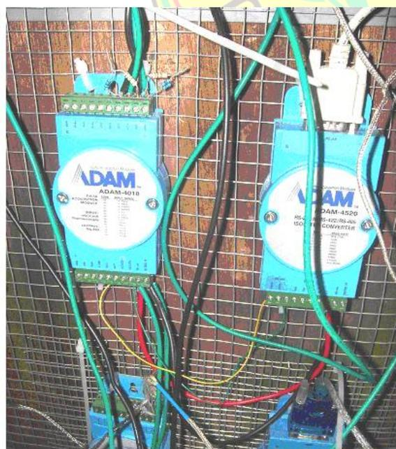
Figure 5. Data acquisition modules
