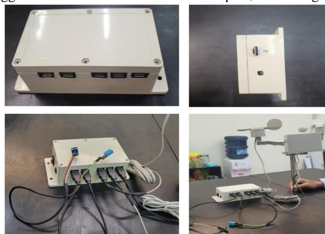
Figure 1. Hardware of data logger.
