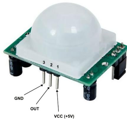
Gambar 3. Passive InfraRed Sensor
