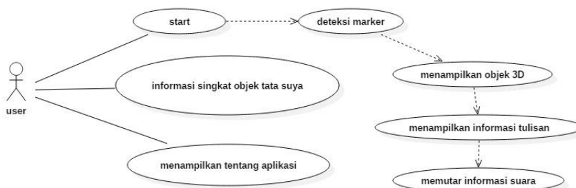
Gambar 3 Use Case Diagram
