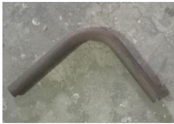
Gambar 9. Hasil Uji As ST 41
