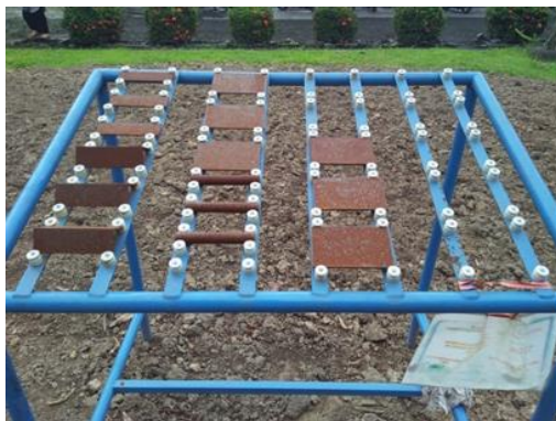
Figure 3. Test Specimens on Measurement Tray (location of palm oil industry of PTPN 1 Tanjung Seumantoh)
