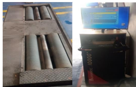
Gambar 3. Alat Uji rem Axle Load Breaker Tester dan Monitor Muller
