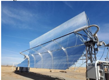
Gambar 1. Kolektor surya tipe parabolic trough (sumber: Dynamic LLC)
