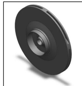
Gambar 6. Rancangan Impeller Condensate Booster Pump 3D
