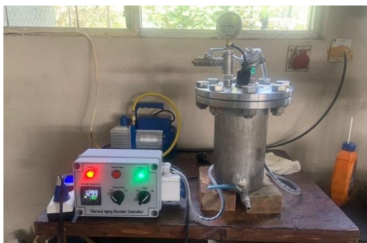
Gambar 1. Tampilan skematis Accelerated Thermal Aging Chamber .
