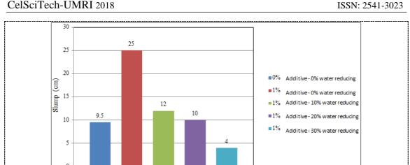
Figure 3. Figure The relation of slump to variation of water on the concrete strength fc'20 MPa
