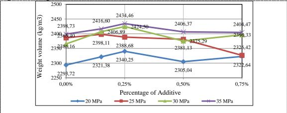
**Figure 4.** Figure The Relatition of weight volume to percentage of BetonMix on the various concrete strength
