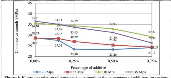
**Figure 6.** Figure the relation of compressive strength to the percentage of additives on various strength
