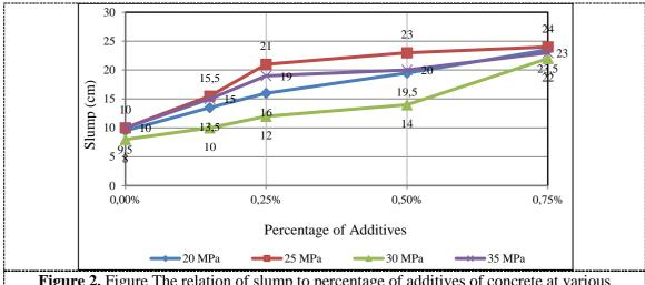
**Figure 2.** Figure The relation of slump to percentage of additives of concrete at various concrete strentgh
